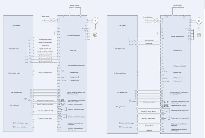
Note: Pulse given and encoder frequency division output are not available for A1/B1 but available for H1.
