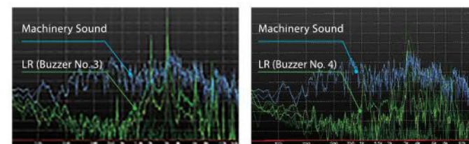
(Buzzer No.3) Rapid Hi-low Sound 2016Hz/3012Hz (Buzzer No.4) Sweep Sound 1000Hz - 4032Hz (changing)
